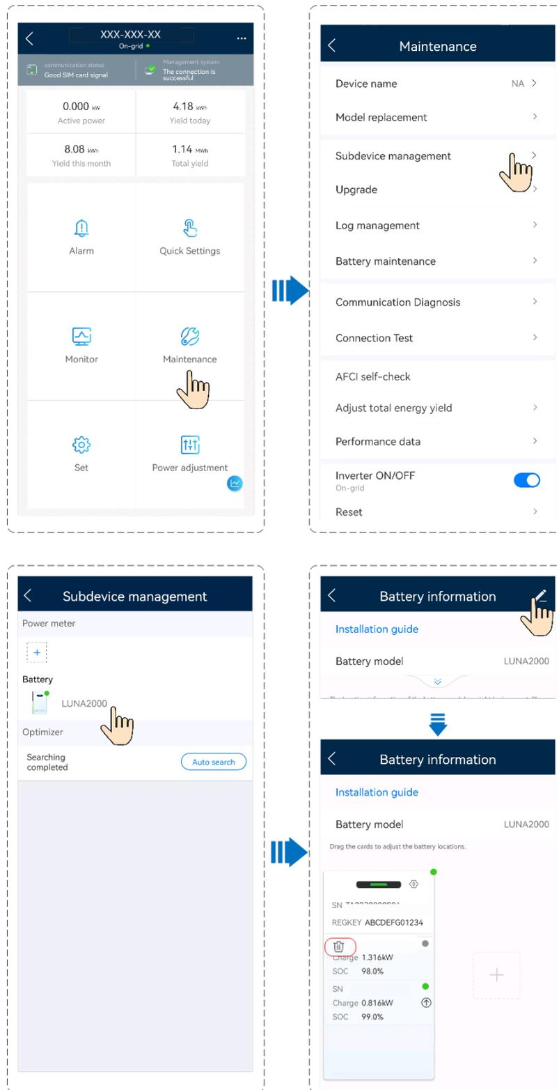
When the EMMA is used for networking, **connect the EMMA on the app**, tap **Monitor** on the home screen, select the connected inverter, choose **Maintenance** > **Subdevice management**, tap the ESS icon, and delete the offline Energy Storage Module.
