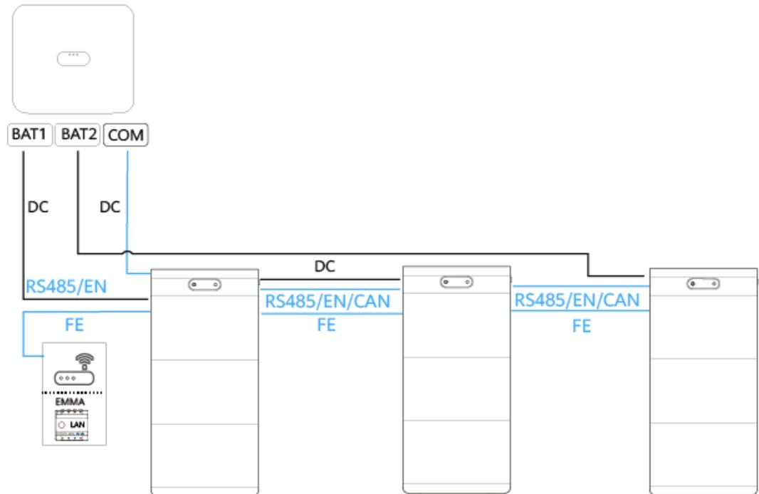
**Figure 2-12** Connecting the ESSs to the inverter (4)
