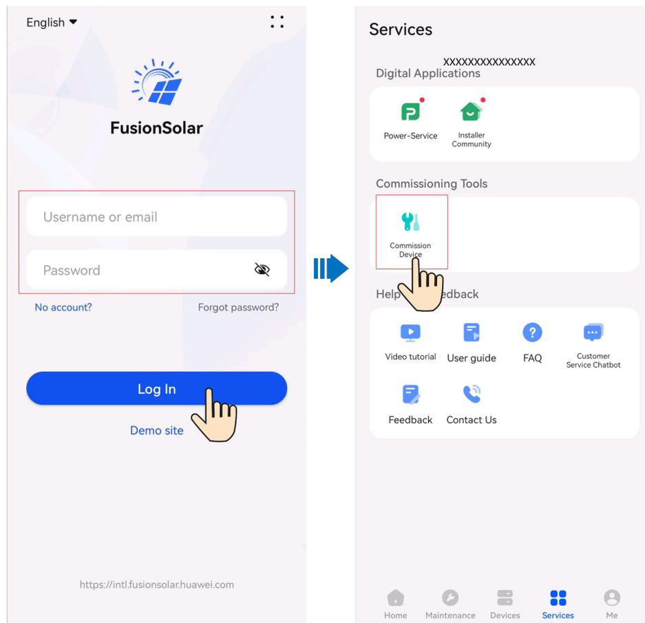
**Step 2** Connect to the inverter WLAN, log in as **Installer**, and access the device commissioning screen.
