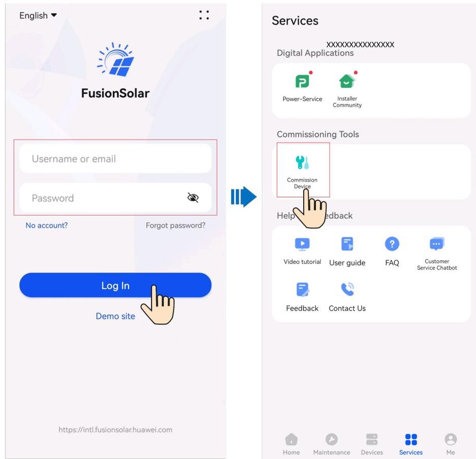
**Step 2** Connect to the EMMA WLAN, log in as **Installer**, and access the device commissioning screen.
