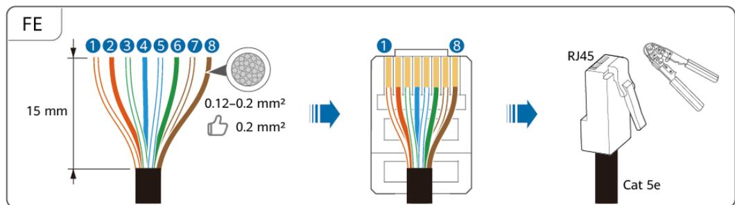
Figure 5-7 Signal port connections
